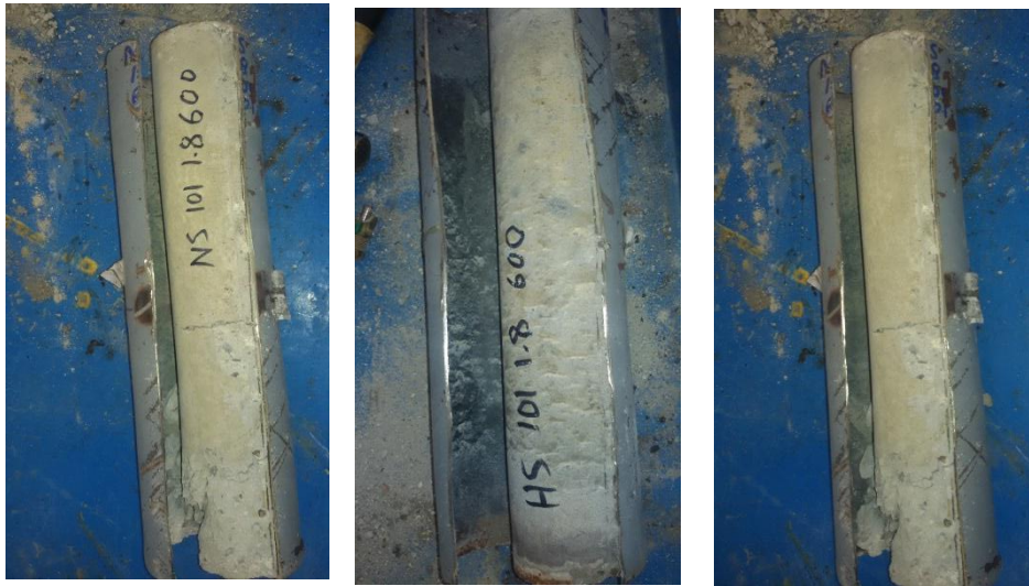
Fig. (9) Crushing of concrete at bulge regions of CFST
